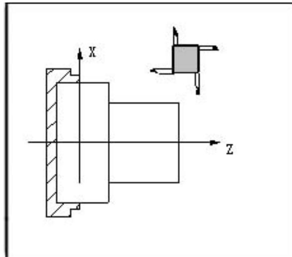
Fig. 1-1-2 Coordinates of Front Tool Holder    Fig. 1-1-3 Coordinates of Rear Tool Holder
