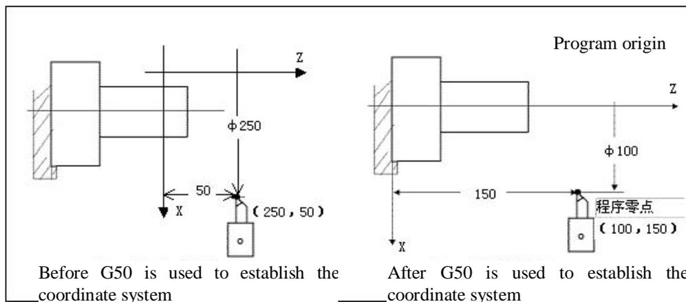
As shown in the above figure, after the instruction segment “G50 X100 Z150” is executed, the workpiece's coordinate system will be established and the point (X100,Z150) considered the program origin.
