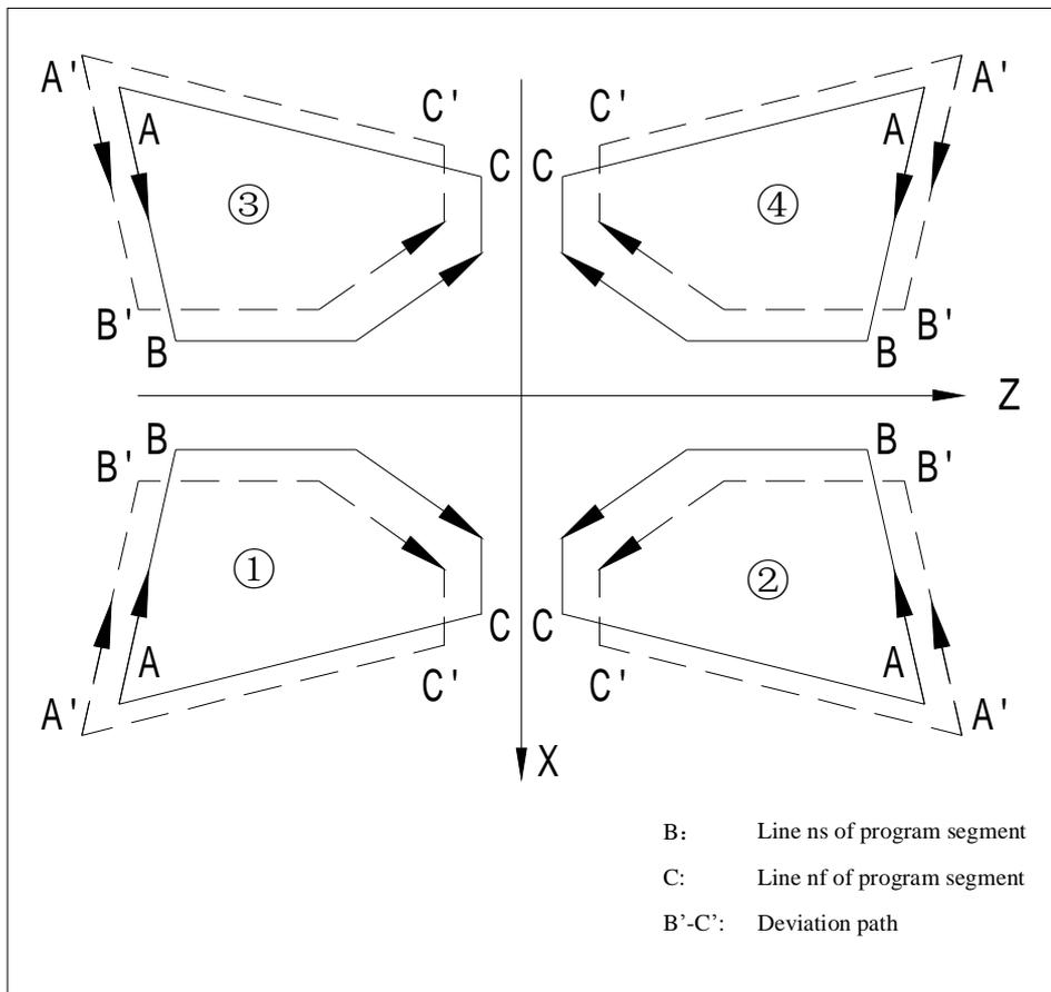
1)  $\Delta i$  can be set through the parameter (116-G73 allowance on axis X), and the set value can be modified through the program instruction. When  $\Delta i$  smaller than  $\Delta u$ , the system will alarm.
