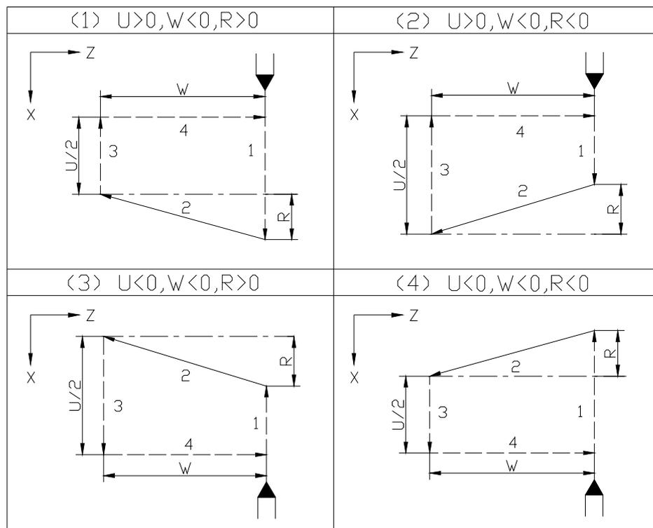
When symbols of R and U are inconsistent with each other, if  $|R| > |U/2|$ , the system will alarm as “1268-G90, G92 and G94 program error”, meaning R value has exceeded the permitted range.
